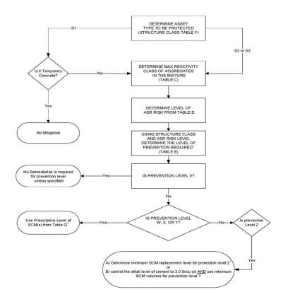
Note 1: The prevention level may be reduced by one level if low alkali cement (≤ 0.70) is used.
