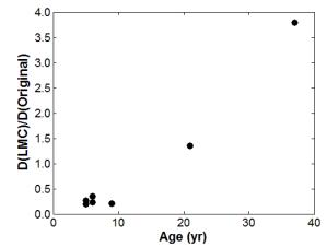
Figure 51. Ratio of diffusion coefficient of LMC overlay to the diffusion coefficient attributed to underlying concrete for the same core
