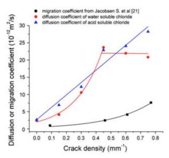
Figure 22. Effect of crack density on the diffusivity of water soluble chloride (WSC) and acid soluble chloride (ASC), 1 mm<sup>-1</sup> = 304.8 ft<sup>-1</sup>, 1 m<sup>2</sup>/s = 10.764 ft<sup>2</sup>/s (Mu et al. 2013)
