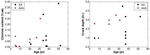
Figure 60. Comparison of chloride content based on concrete type for off-crack locations
