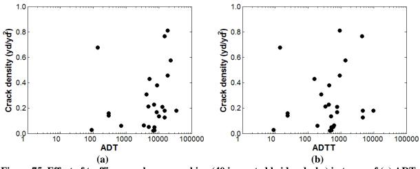
Figure 75. Effect of traffic on early-age cracking (40 inspected bridge decks) in terms of (a) ADT; (b) ADTT
