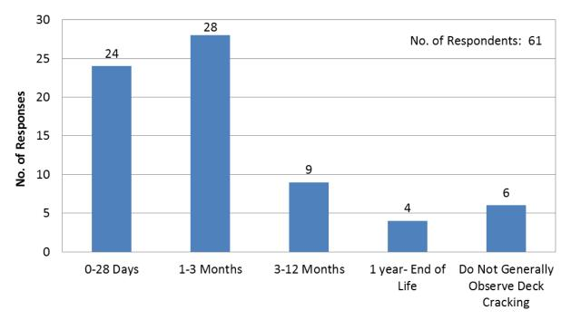
Figure 37. Respondents Observations of Initial Cracking
