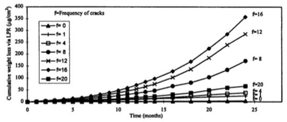
Figure 15. Effect of crack frequency on the cumulative weight loss due to corrosion based on linear polarization resistance (LRP) test,  $1 \mu g/cm^2 = 0.1422 \mu lb/in.^2$  (Arya and Ofori-Darko 1996)
