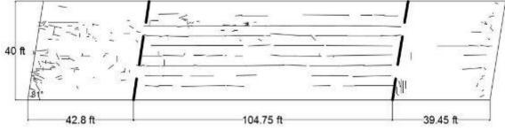
Figure 102. Bridge 5081 crack map
