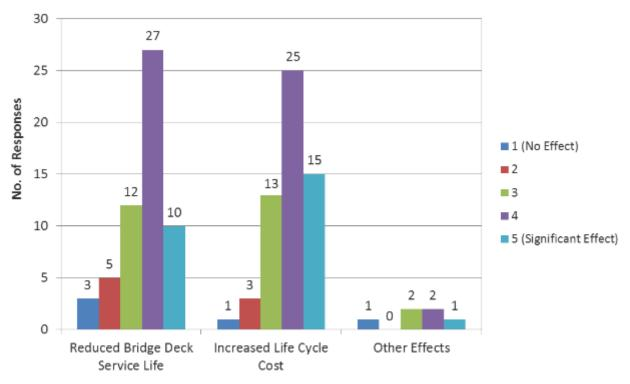
Figure 41. Effect of Early-Age Cracking on Bridge Deck Long-Term Performance
