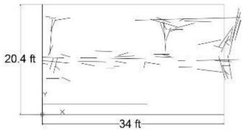
Figure 119. Bridge 30752 crack map
