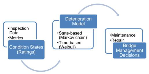
Figure 24. The role of deterioration models in bridge management systems
