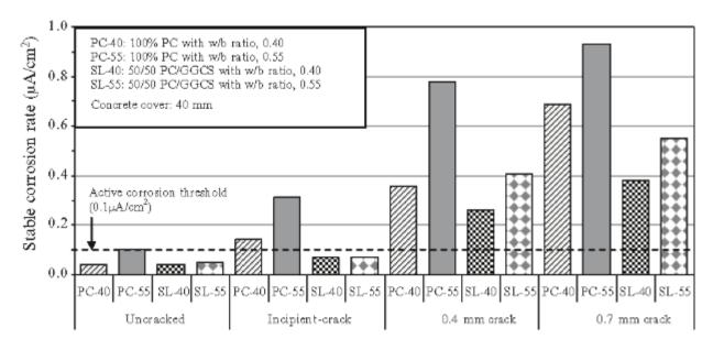
Figure 13. Effect of concrete quality and crack width on steel corrosion rate for PC (portland cement) and GGCS (ground granulated Corex slag) concrete specimens (Otieno et al. 2010a,b)
