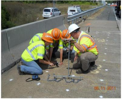
Figure 94. Inspectors conducting chain drag on deck. (FHWA 2013)
