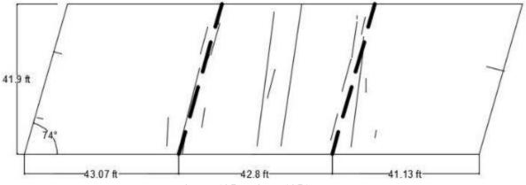
Figure 105. Bridge 12517 crack map
