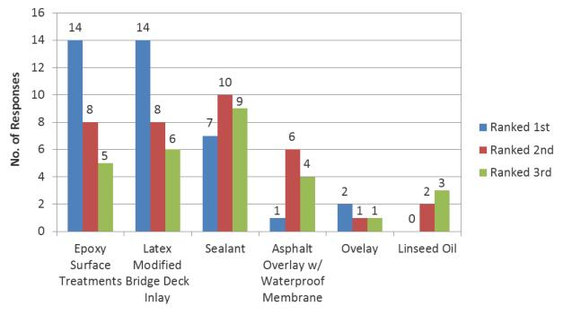
Figure 44. Ranking of the Remediation Methods
