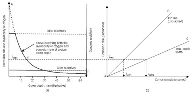
Figure 16. Schematic diagram of the relationship between corrosion rate, oxygen availability and resistivity, to account for crack width (PC: ordinary Portland cement, SCM: supplementary cementitious materials) (Otieno et al. 2010a)
