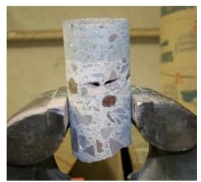
Figure 46. An example of a core with drill holes at the rebar level.
