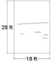
Figure 97. Bridge 251 crack map
