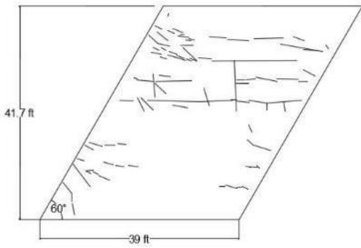
Figure 101. Bridge 4908 crack map
