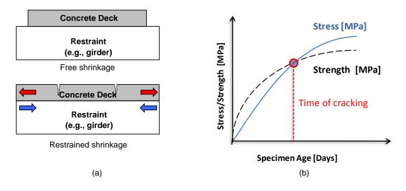
Figure 2. (a) Schematic illustration of shrinkage-induced cracking in concrete bridge decks; (b) Time-dependent stress and strength development in concrete, leading to early-age cracking
