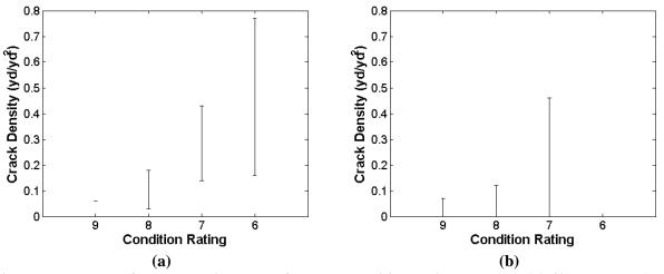
Figure 77. Ranges of crack density values for each condition rating based on (a) 40 deck data (nonoverlayed); (b) 163 deck data.
