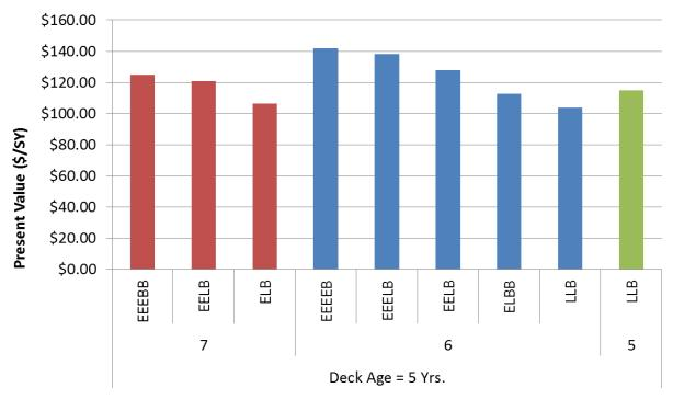
Figure 92. Treatment Sequences and Life Cycle Costs for a BPN 1&2 Bridge with Deck Age of 5 Years
