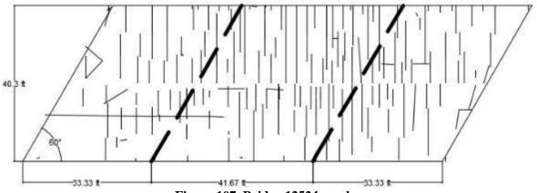
Figure 107. Bridge 12524 crack map
