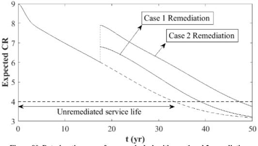
Figure 90. Deterioration curve for example deck with case 1 and 2 remediation
