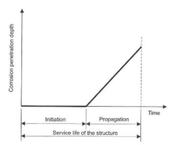
Figure 7. Initiation and propagation phases for corrosion in reinforced-concrete structure (Tuutti 1982)
