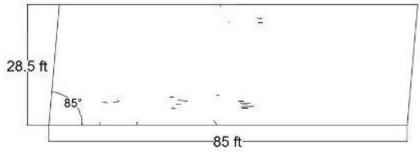
Figure 103. Bridge 6457 crack map
