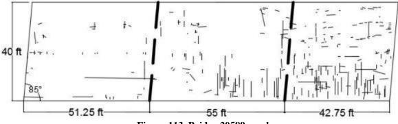
Figure 113. Bridge 20589 crack map
