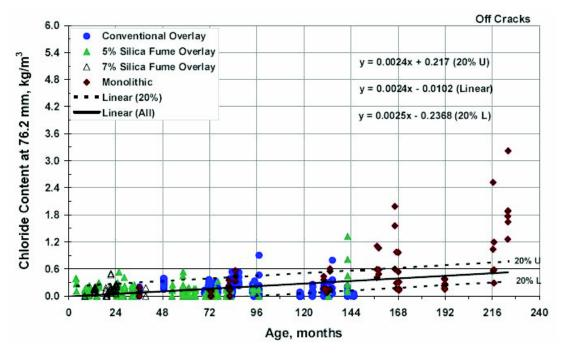
Figure 10. Chloride content at the rebar level (3.0in = 76.2mm) taken from uncracked regions of bridge decks versus age, 1kg/m<sup>3</sup>=1.69 lbs/yd<sup>3</sup>. (Lindquist et al. 2005)
