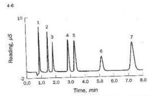
Figure 4110:1. Typical Inorganic anion separation. Eluent: 1.7 snM NaHCO<sub>5</sub>, 1.8 nM NaCO<sub>5</sub>; sample loop: 25 µL; flow rate: 2.0 mL/min; column: Dionex AG4A-SC plus AS4A-SC.
