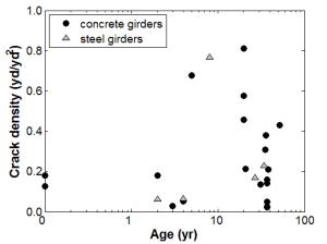
Figure 63. Crack density in terms of girder type (40 inspected bridge decks)
