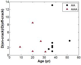
Figure 59. Ratio of diffusion coefficient for on-crack to off-crack cores
