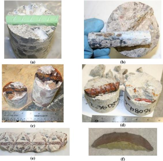
Figure 48. Examples of (a) a completely intact epoxy-coated rebar (Core C2\_4908\_NC); (b) a rebar with minor corrosion; (c) an extremely corroded black rebar (Core C1\_20506\_C); (d) a corroded epoxy coated rebar (Core C2\_36084\_C, 37 year old deck); (e) rebar sample No. 1 for which percent effectiveness was approximated(Core C1\_652\_NC); (f) rebar sample No. 2 for which percent effectiveness was approximated (Core C1\_12905\_C)
