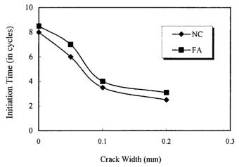
Figure 12. Initiation times (time to start of propagation phase) for cracked NC (normal cement) and FA (fly-ash blended) concrete beams, 0.1 mm = 0.00394 in. (Li 2001)
