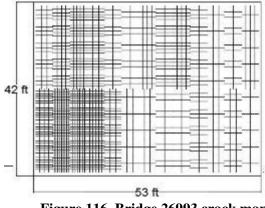
Figure 116. Bridge 26993 crack map
