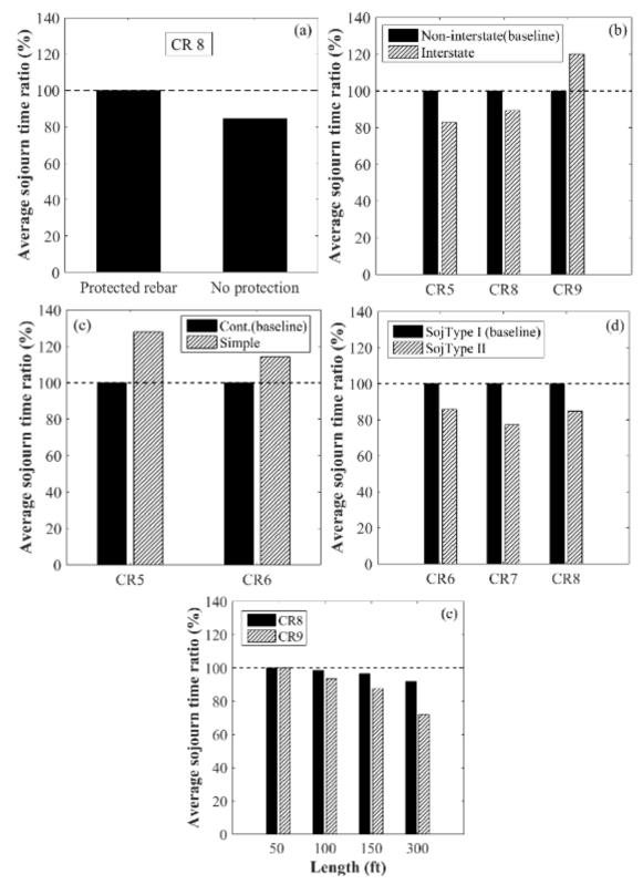
Figure 84. Ratio of average expected sojourn time to the baseline average expected sojourn time based on (a) Whether the rebar is protected or not; (b) Whether the deck is located on an Interstate or Non-interstate; (c) The type of span interaction; (d) Type of sojourn time. Dashed lines on figures represent baseline
