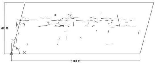
Figure 118. Bridge 30700 crack map
