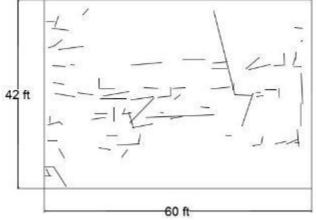
Figure 117. Bridge 30643 crack map
