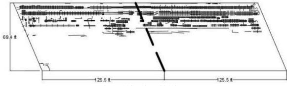
Figure 114. Bridge 20613 crack map
