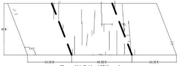
Figure 106. Bridge 12518 crack map
