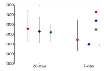
Figure 55. Average (data points) and range (error bars) of compressive strength for each concrete type at 28 and 7 days (163 new bridge decks)
