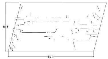
Figure 115. Bridge 21651 crack map
