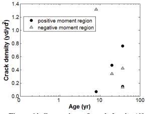
Figure 64. Comparison of crack density (40 inspected bridge decks) for positive and negative moment regions
