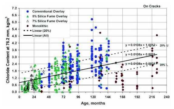
Figure 11. Chloride content at the rebar level (3.0in = 76.2mm) taken from cracked regions of bridge decks versus age, 1kg/m<sup>3</sup>=1.69lbs/yd<sup>3</sup> (Lindquist et al. 2005)
