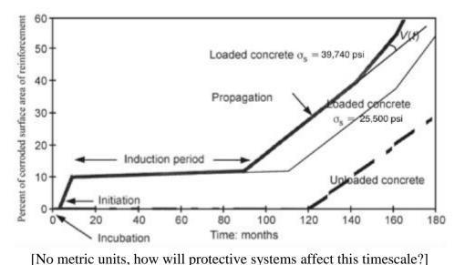
Figure 9. Schematic modeling of the corrosion process for cracked (loaded) and un-cracked (unloaded) concrete, (Francois and Arliguie 1994, Tuutti 1982)
