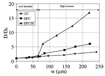
Figure 20. The effect of crack width on the ratio of diffusion coefficient of cracked concrete to uncracked concrete (D/D<sub>0</sub>). The results are shown for OC (ordinary concrete), HPC (high performance concrete) and HPCSF (high performance concrete containing silica fume) 100  $\mu m = 0.004$ in. (Djerbi et al. 2008)
