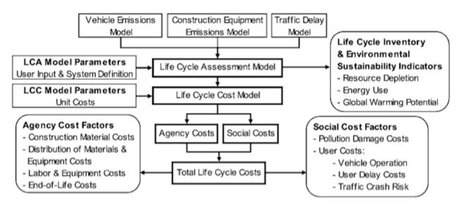
Figure 33. Integrated LCA-LCCA model flow diagram (Kendall et al. 2008)
