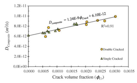
Figure 21. Estimated diffusion coefficient of cracked samples ( $D_{composite}$ ) as a function of crack volume fraction, 1 m<sup>2</sup>/s = 10.764 ft<sup>2</sup>/s (Akhavan and Rajabipour 2013)
