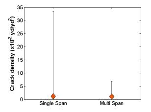
Figure 65. Comparison of average (data points) and range (error bars) of crack density at initial inspection (163 new bridge decks) between single and multi-span bridges
