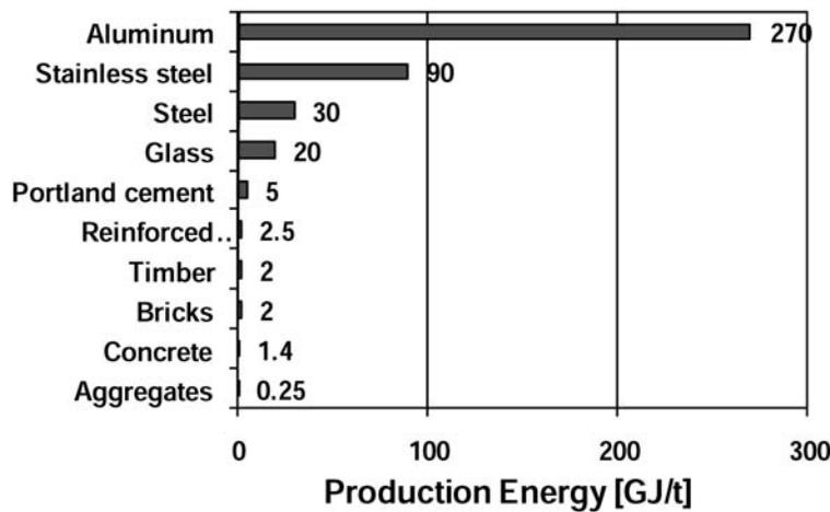
**FIGURE 2.** Energy of production for common building materials.
