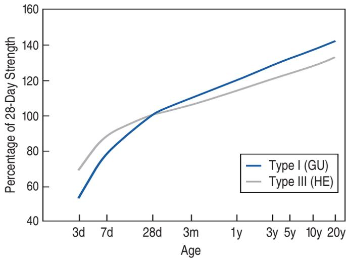
**Figure 2. Representation of concrete strength gain with age for two different cement types. (Ref. 9)**
