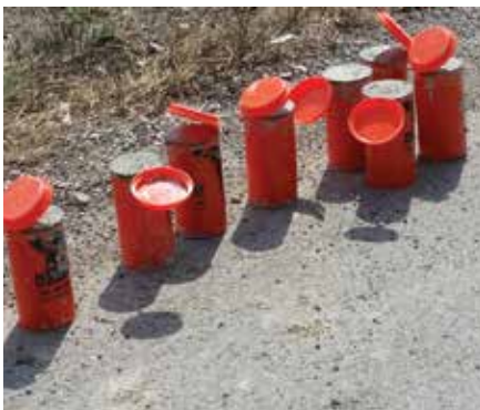
Fig. 2: Examples of initial curing conditions that do not comply with ASTM C31/C31M. 2 High temperature and moisture loss at the critical early age will lead to reductions in later-age strengths, even if standard curing is provided subsequently
