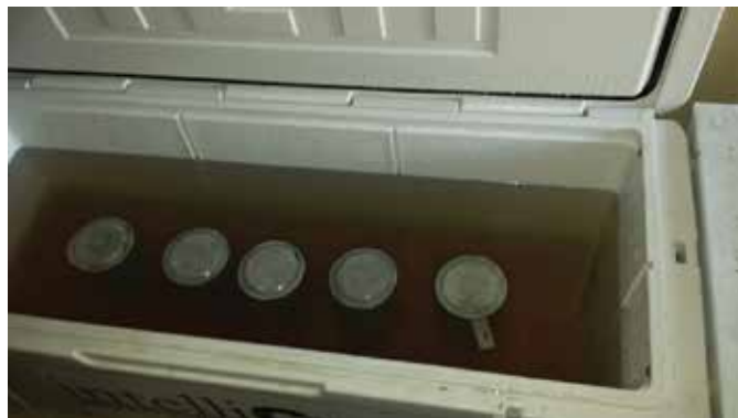
Fig. 3: Example of a thermostatically controlled curing container with specimens stored under water. If the unit is functioning as specified, initial curing will meet the requirements of ASTM C31/C31M
